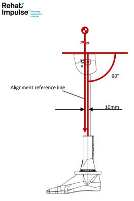
The prosthetic foot should be aligned according to the manufacturer's recommendation (as a general rule an external rotation of 5-7° is recommended). An incorrect initial position can lead to inappropriate force transfer from the ground to the prosthesis.
